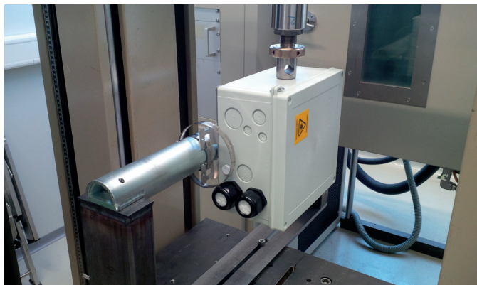
Figure 3 – Pole-mounted box with fixture in tensile & compression test rig for lateral load application during testing
