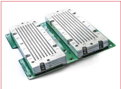
▲ Fig. 4 Terragraph RF front-end board. Two antennas were used for transmitting (Tx) and receiving (Rx), respectively.
