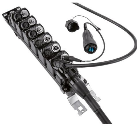
Hybrid cables of HUBER+SUHNER combine optical fiber and DC power, are highly flexible and easy-to-route. Two rip cords between the shielding and the jacket allows a quick stripping of the jacket. The shielding, a copper foil under the jacket and the drain wire maintain contact throughout the cable run and allow potential equalisation and a safe installation with regard to lightning strikes.
