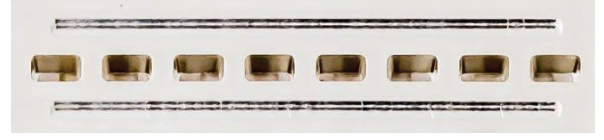
Fig. 3. Fabricated prototype. Grooves are visible above and below the horn antennas.
