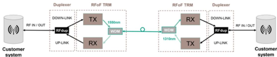
Using intensity modulation of optical laser light by RF signal amplitude ensures that the analogue characteristics of the RF signal are retained from end to end.
