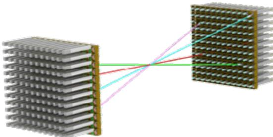
The patented POLATIS® DirectLight™ high-performance switching technology from HUBER+SUHNER, minimizes impairments to RF signals traversing the switch connections.
