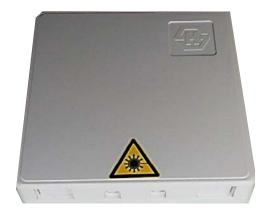
This outlet has been designed for the FTTH market to terminate the optical network and the indoor subscriber side. It is the passive interface before the ONT. The outlet is composed of an equipped base and a cover. Is provided complete with two 40mm splice protections and fixing elements.
