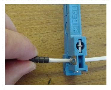
Feed the loose tube through the cable ties so that the loose tube can be removed.
