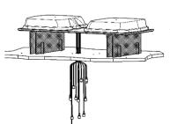
Use parts of the packaging to easily position the antenna above the cable breakthrough as indicated on the picture.
