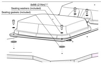
1) For a minimum 8mm thick contact surface, use screws with a minimum length of 18mm.
