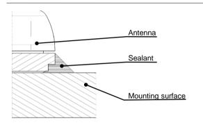
It is optional to seal the perimeter of the antenna with sealant.
