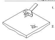
Clear the area where the antenna is mounted from paint, corrosion or any anodized layer.
