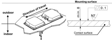
The mounting surface shall be planar and stable. The material of the mounting surface shall be steel or aluminium.
