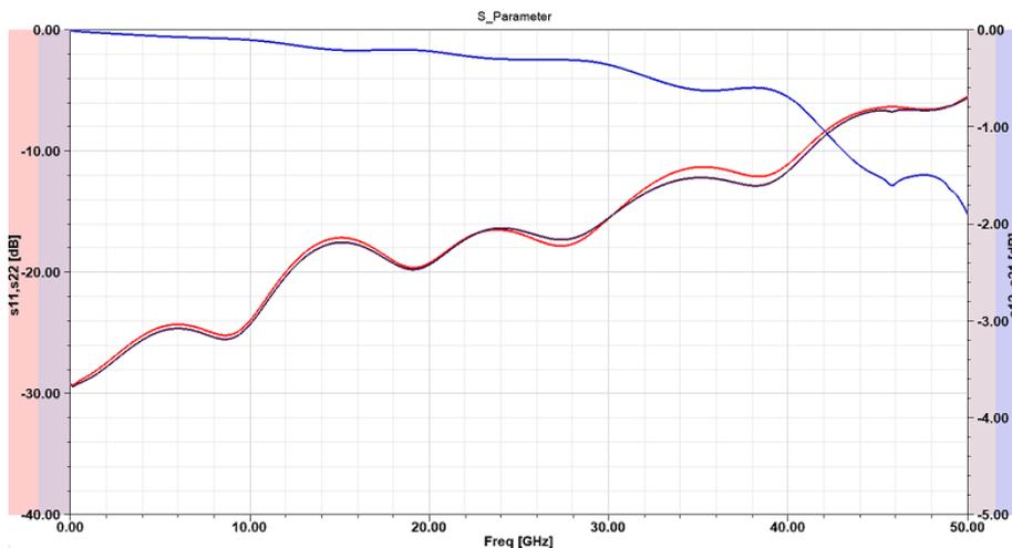
*Graph 6: Simulated S-parameters of footprint C (non-optimized).*
