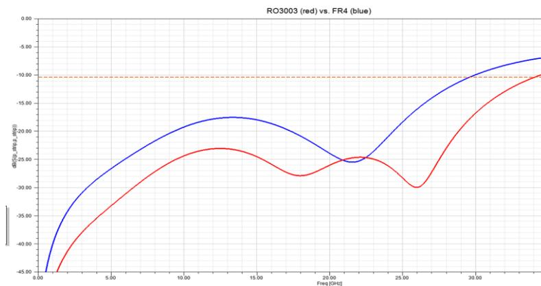
*Graph 3: Simulated S11 results (up to 35GHz): Simulation A (RO3003) in red. Simulation B (FR4) in blue.*
