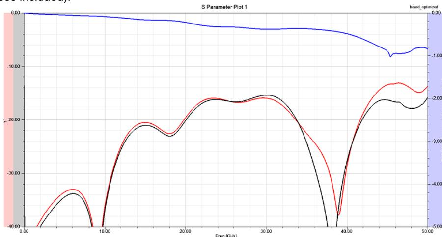
**Graph 9: Simulated S-parameters of optimized footprint D (optimized)**
