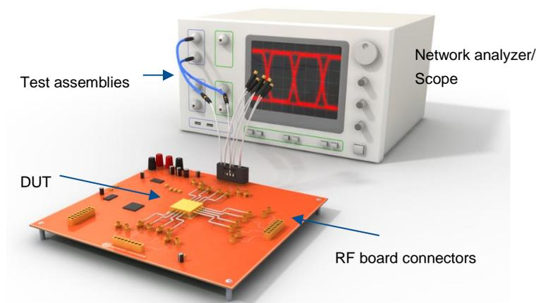
*Fig.1: Standard test setup for Design Validation Testing (DVT) with network analyzer and/or scope*
