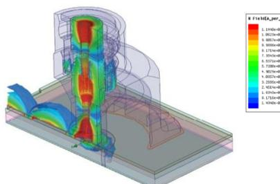
*Graph 2: Representation of H-Field transitioning from a coaxial board connector onto a microstrip*
