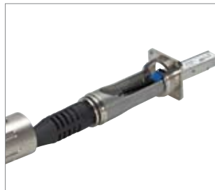
Remove LC dust caps and plug LC duplex connectors into SFP module
